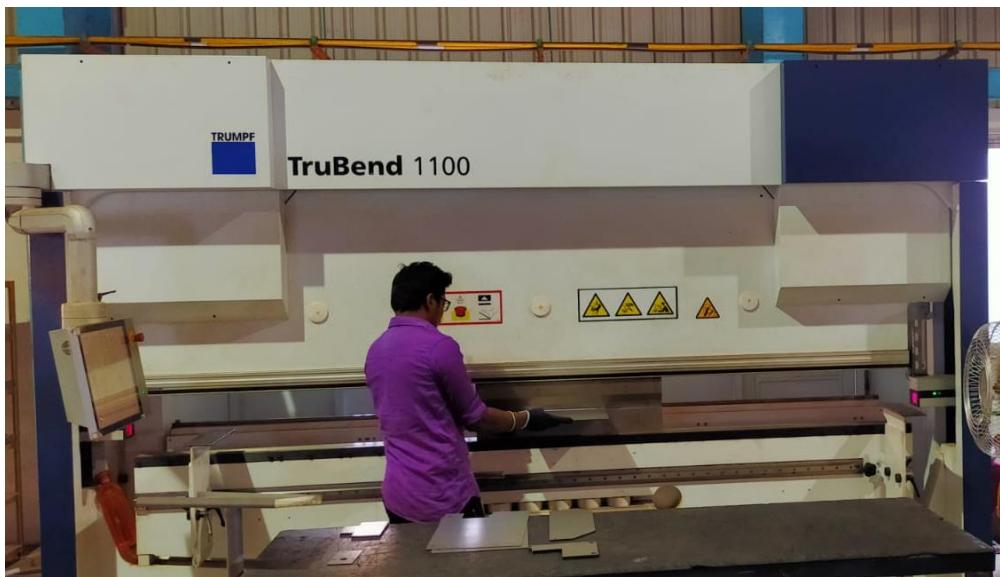
**TRUMPF HYDRAULIC PRESS BRAKE 100 T WITH AUTO CROWNING**
